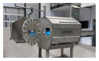
The swivel arm for easily replacing the cutting disks. Here, hollow spaces were eliminated, and the number of screw fastenings was reduced. It also features a new function for fixing the carriage that allows the cutting disk to be moved back and forth, thus further improving operational safety.
