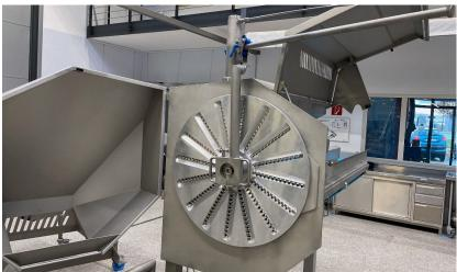
The swivel arm is an important optional accessory for the GS 20 belt cutting machine, which is used to easily replace the cutting disks.
