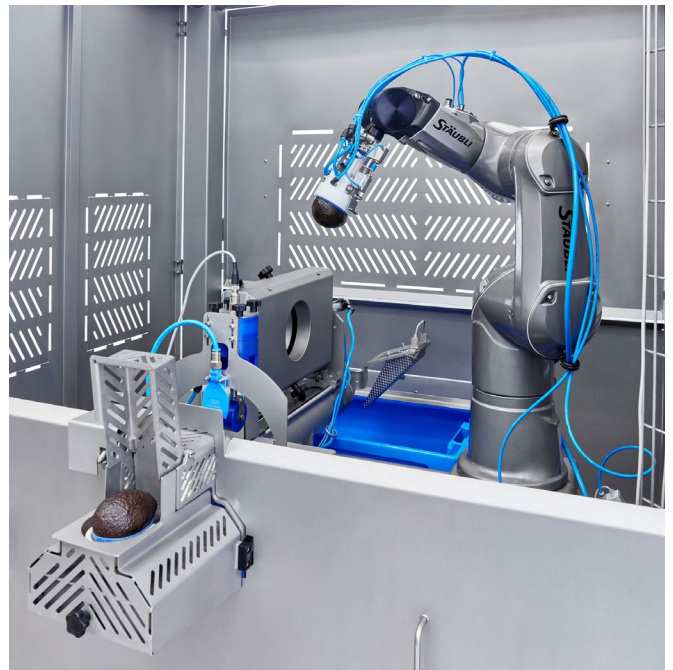
▼ Along with its pitting and peeling unit, the Avocado Robot Line (below) also features a grabber specially adapted to handle the shape and texture of avocados.
